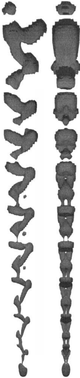
FIG. 10. Flow past a sphere at Re = 300 . XY view (side) and XZ view (top) of the complete extent of the vorticity structures (identified by the \lambda_2 method) at T = 75 .
